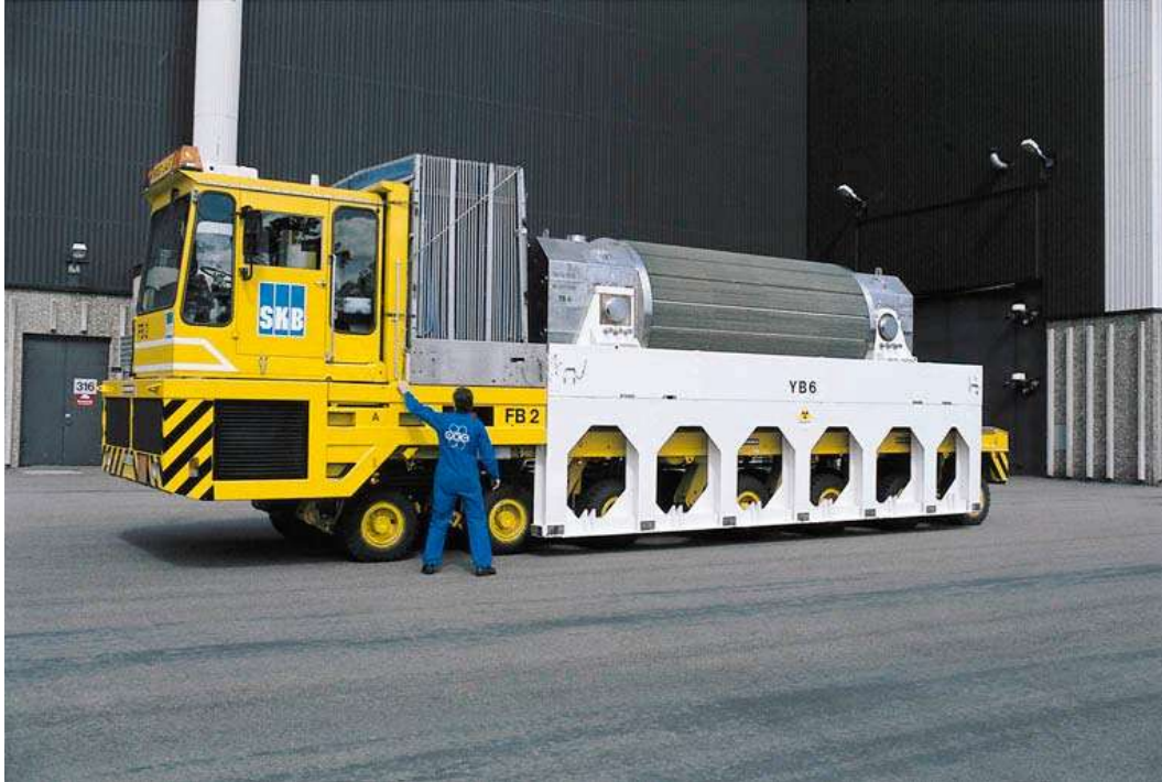
Figure 8.3. Transport cask for spent nuclear fuel.
