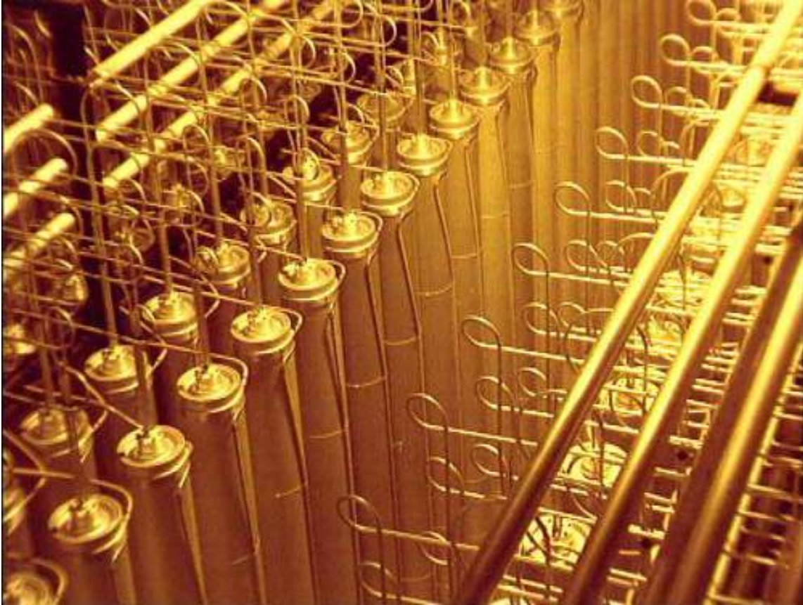
Figur 4.3. Cascaded centrifuges, which can run maintenance free for more than 10 years. This method is energyware efficient, consuming approximately 0.1% of the electricity generated.
